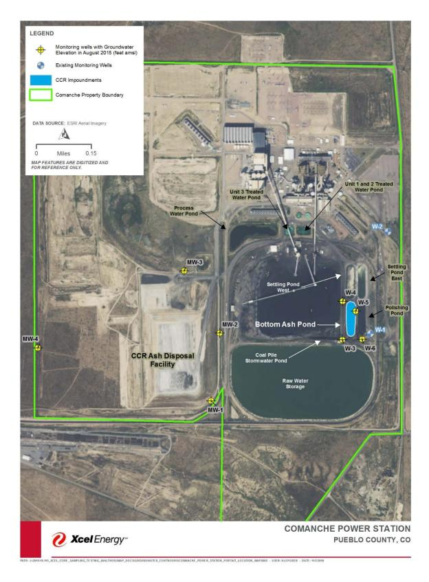
Figure 2. Comanche Station – CCR unit and monitoring well location map.
